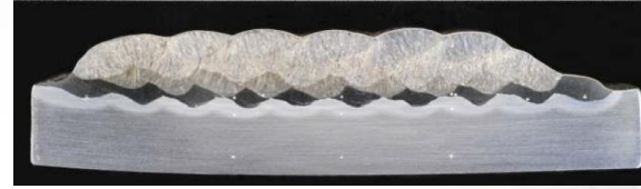
Weld Overlay Bond
