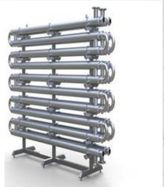
A double pipe heat exchanger, into its simplest form is one pipe within another larger pipe. One fluid flows through the inside pipe and the other flows through the annulus between the two pipes. The wall of the inner pipe is the heat transfer surface.
