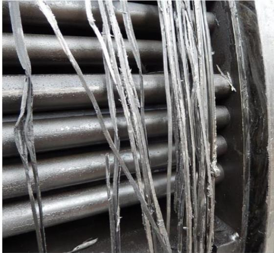
SW Gaskets are not reliable and break apart under high assembly loads
