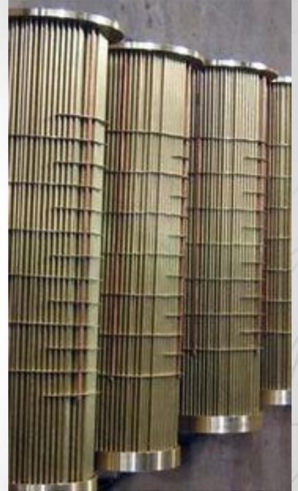
A fixed tube-sheet heat exchanger has straight tubes that are secured at both ends to the tube-sheets welded to the shell.
