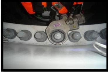
Hydraulic Bolt Tensioning Example
