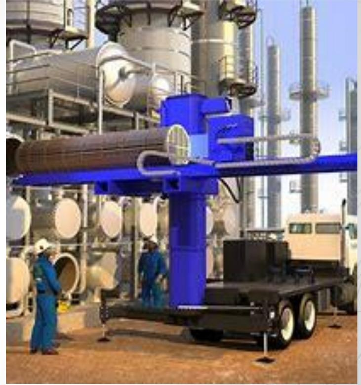
Must use outriggers and bundle weight not to exceed 25 tons on Truck Mounted extractor and must follow length and diameter specifications.
